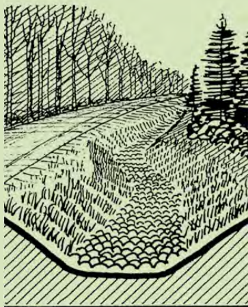
Grass and stone stabilized ditch
