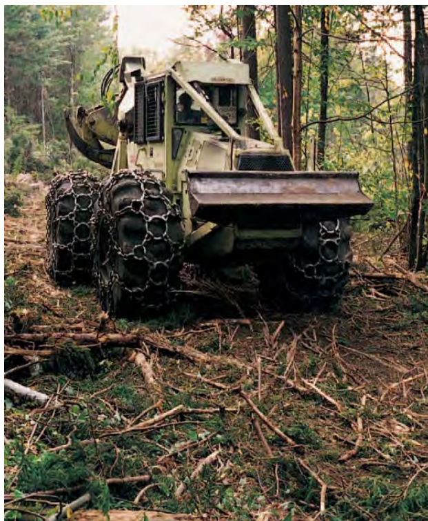
Brush on skid trails, as well as frozen ground, helps minimize soil disturbance and rutting.
